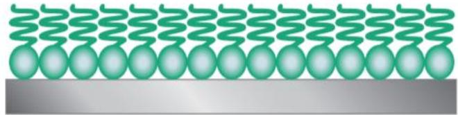
Fig2 Protective shield 50 – 200 angstroms deep prevents moisture and gases from reacting with metal components
