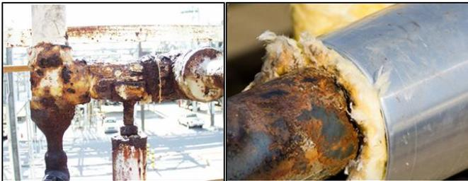
Fig1 Corrosion paint failure & CUI Damage on a Steam piping
