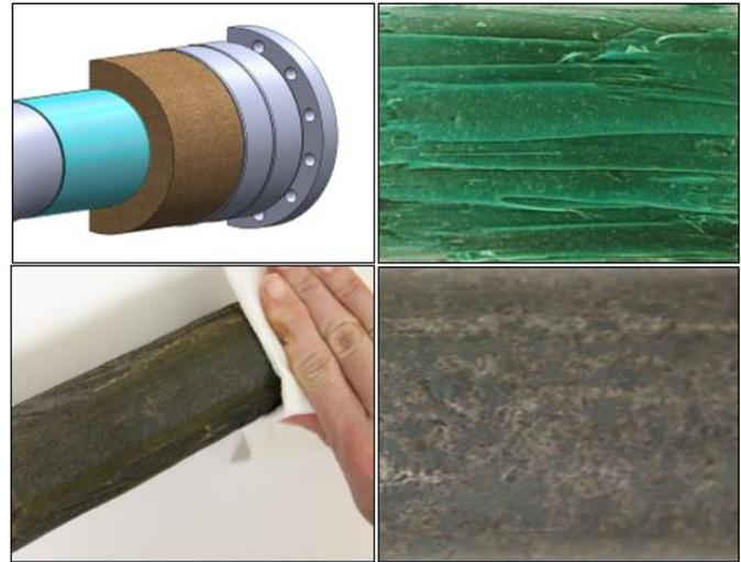
Fig3 Application and Visual Inspection Results. Zero indications of corrosion reactions.
